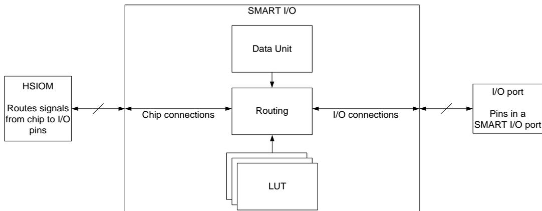
There are several areas in the GUI to configure signals: Chip, I/O, Data Unit, and LUT. Inputs to the chip from the I/O port can be logically operated upon before being routed to the peripheral blocks and connectivity of the chip. Likewise, outputs from the peripheral blocks and internal connectivity of the chip can be logically operated upon before being routed to the I/O port.
