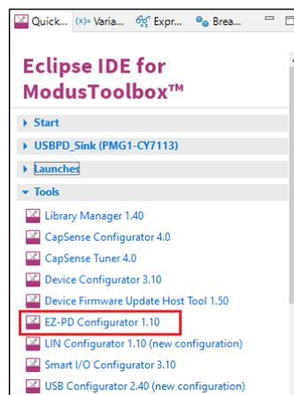
Similar to the make command method, launching the EZ-PD™ Configurator using the Eclipse IDE opens the tool for the selected application. Refer to the [Eclipse IDE for ModusToolbox™ user guide](#) for details about the IDE.
